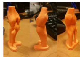
Dog knee printed by JuggerBot with FibreTuff biopolymer
